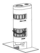
Turn off the LED when finished by pressing the LED button ②.
