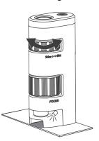
Rotate the focusing ring (5) until the image is sharp and clear.
