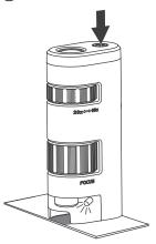
Adjust the zooming ring 4 to the desired level of magnification.
